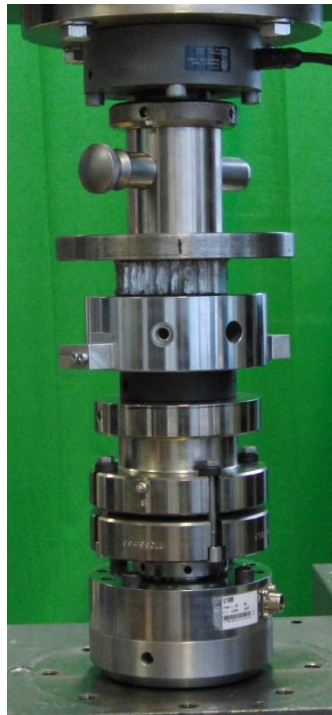
Figure 4.3. ASTM C365 Honeycomb flatwise compression test setup
