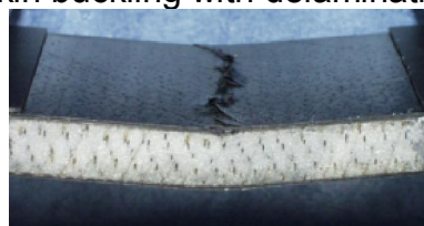
Figure 5.8. Upper skin compression failure in 4-point bending [64]
