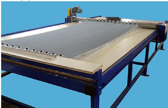
Figure 3.6. Aluminium honeycomb expansion machine [121]
