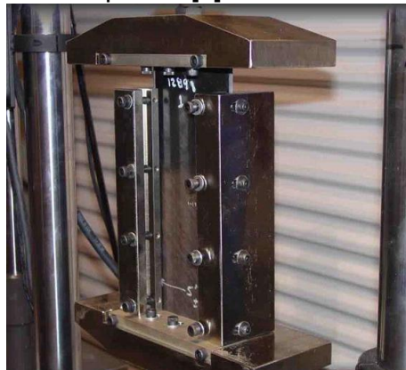
Figure 5.7. NASA compression after impact test setup, [152]
