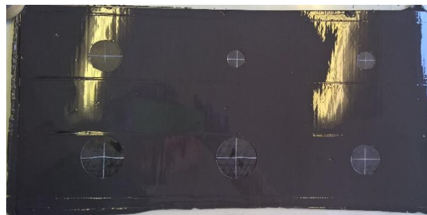
Figure 2.5. Artificial debonding (absence of adhesive layer).
