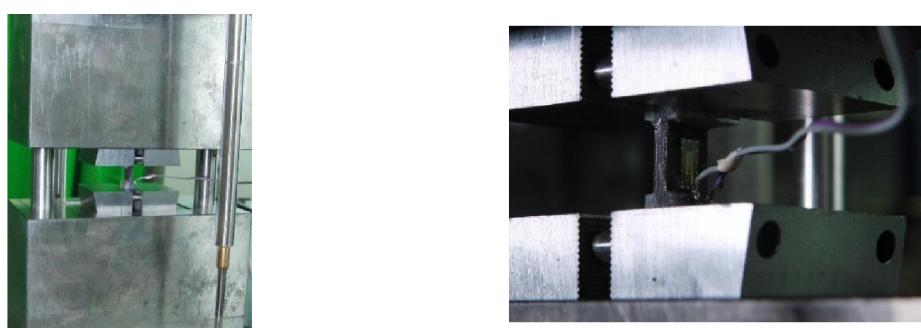
Figure 3.5. 0° direction compression test setup
