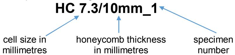
Figure 4.2. Honeycomb specimen labelling example
