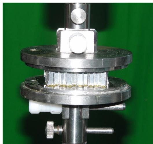
Figure 5.1. Flatwise tension test setup
