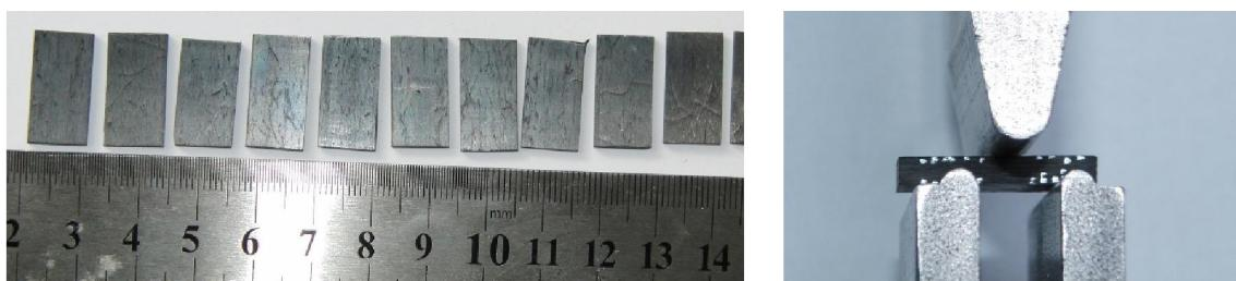
Figure 3.16. Specimens (a) and test setup (b) of short beam shear test
