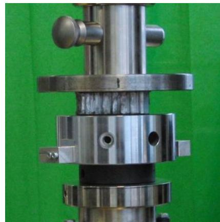
Figure 4.5. Flatwise compression test setup
