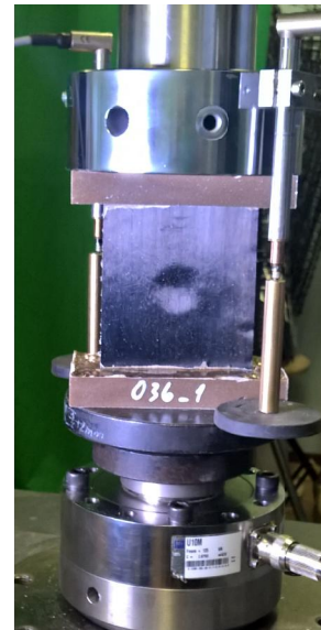
Figure 8.9. Edgewise compression test
