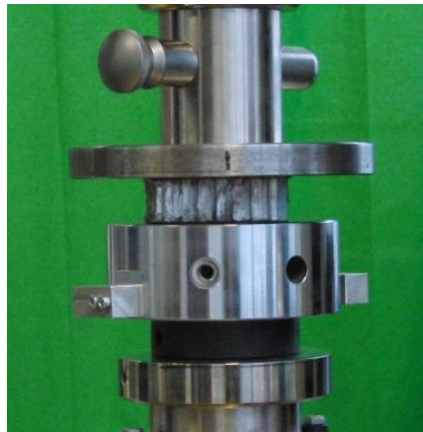
Figure 5.4. Flatwise compression test setup
