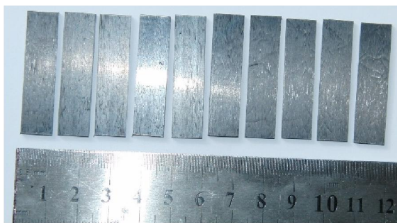
Figure 4.14. Specimens (a) and test setup (b) of short beam shear test with coupon on its lateral side
