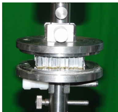
Figure 7.1. Flatwise tension test setup
