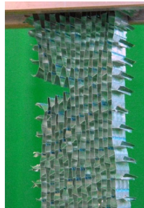
Figure 5.5. Tensile node bond strength test setup and typical failure
