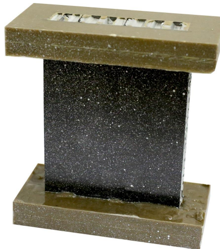
Figure 8.12. Sandwich panel specimen with reinforced ends for edgewise compression
