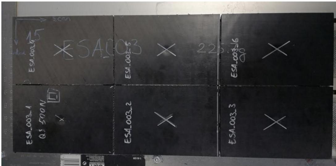
Figure 5.3 Panel cut to individual specimens.
