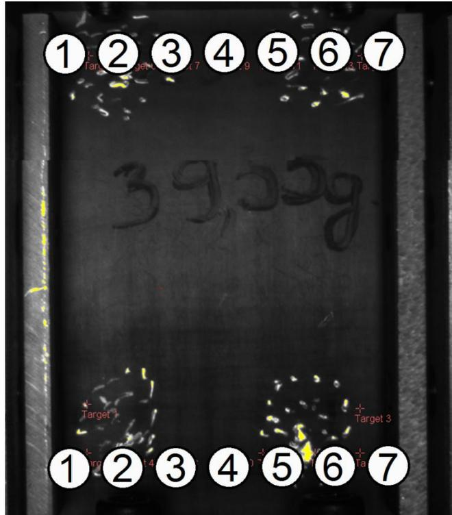
Figure 5.4 Strain distribution measurement along the panel width.
